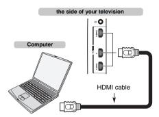
If connecting a PC with DVI terminal, use an HDMI-to-DVI adaptor cable.
